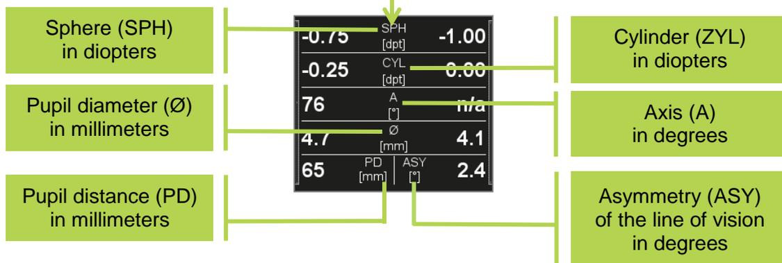
In addition to the measurement values, a measurement result is displayed:
