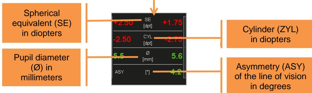
If the measurement values are outside the measuring range, “HYP” (for hyperopia) or “MYO” (for myopia) is displayed as the measurement of the spherical equivalent instead of a quantitative numerical value.
