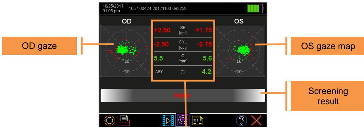
Figure 3: Viewing the measurement values
