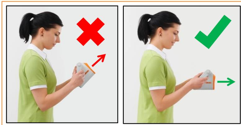
Figure 5: Aligning the plusoptiX 12 model
