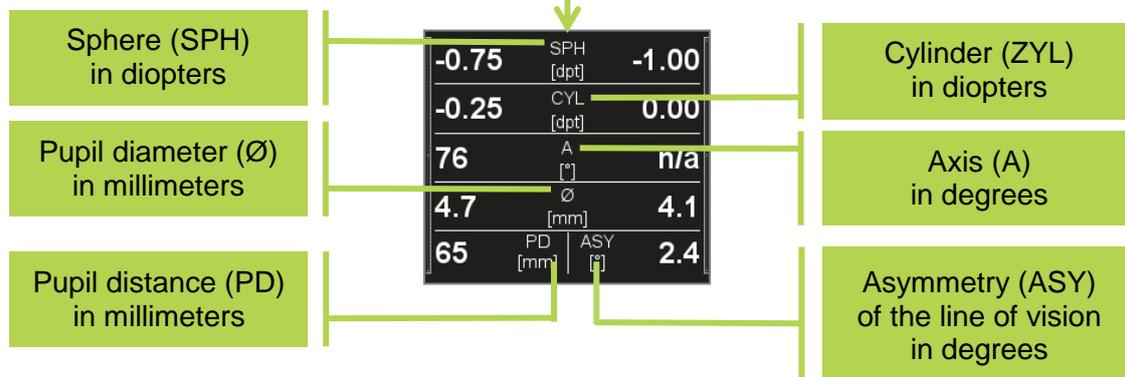
If the measurement values are outside the measuring range, “HYP” (for hyperopia) or “MYO” (for myopia) is displayed as the measurement of the spherical equivalent instead of a quantitative numerical value.
