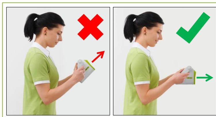
Figure 3: Aligning the plusoptiX A12 model
